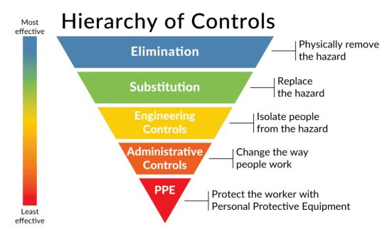
Pictured above is a graphic from OSHA that displays the relationship of the hierarchy of controls.
