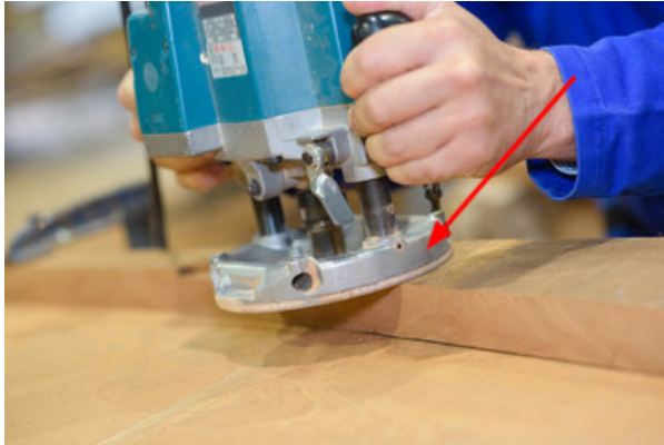
Fixed guard on handheld router
