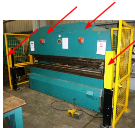
Safety light curtain and two-hand controls
