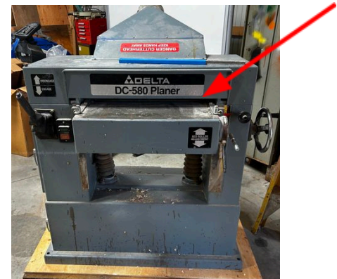
Cutter head is enclosed with a metal guard or a cage.
