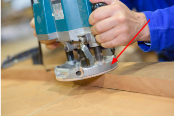
Fixed guard on handheld router
