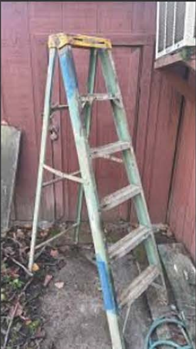
UV damage, decals missing or illegible
