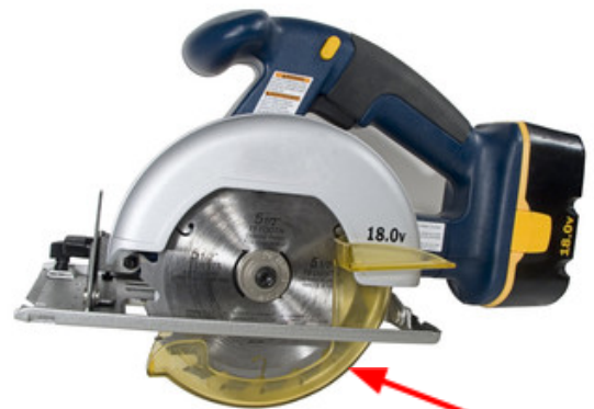
Guarded blade on circular saw
